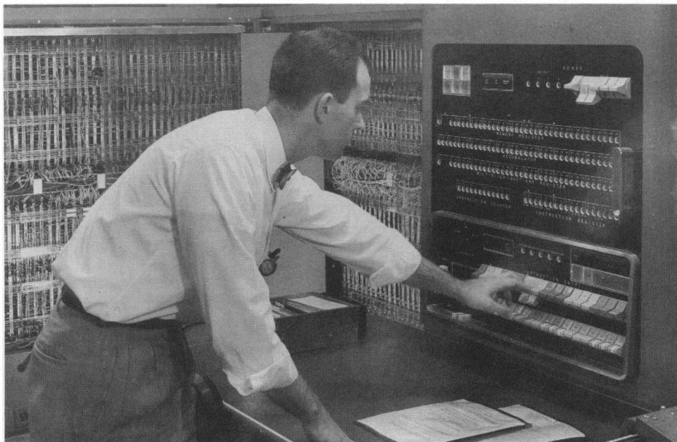
Mathematical Analyst Keith Kersery loads jet transport flutter problem into one of Lockheed's two 701's. On order: two 704's to help keep Lockheed in forefront of numerical analysis and production control data processing.
